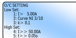
Actual LCD presentation when adjustable parameters are displayed. Screen example above also shows the default settings for OVERCURRENT.
